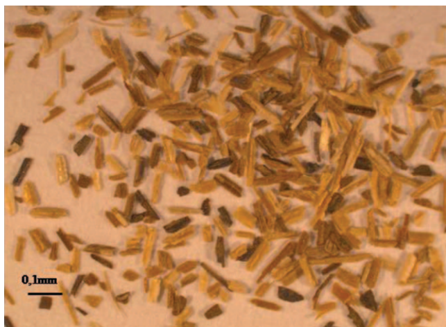
Figure 4. Photomicrograph showing morphology of heart-of-peach palm sheath waste residue. [Color figure can be viewed in the online issue, which is available at wileyonlinelibrary.com .]
